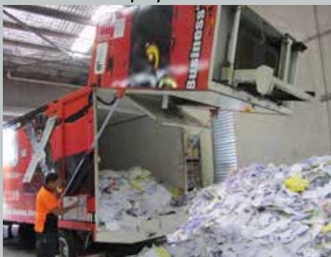
Unloading with concealed lifter
