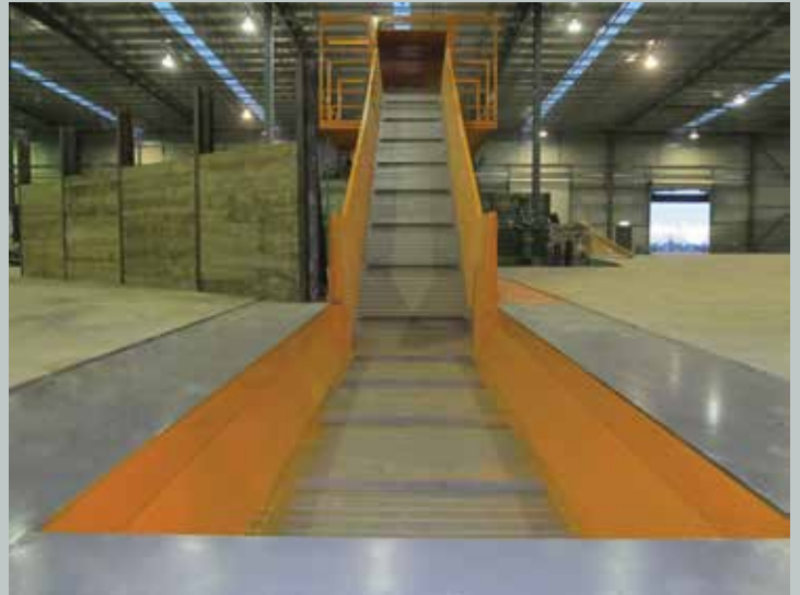
Below ground with 10 metre horizontal feed section deep pit design. 1800mm wide live width x 28 deg incline curved head section. 5mm slats with 65,000LB chain.
