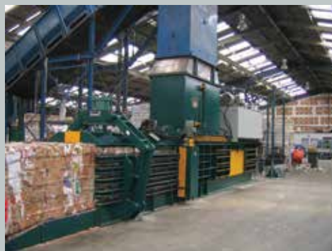
Below Ground with horizontal feed section and secondary horizontal sort section. 1800mm wide live width x 28 deg incline curved head section.
