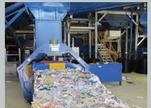
Below ground with 10 metre horizontal feed section deep pit design. 1800mm wide live width x 28 deg incline curved head section. 5mm slats with 65,000LB chain.
