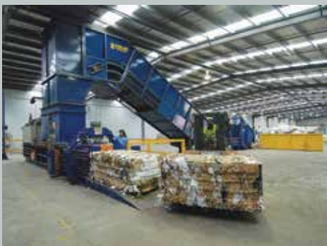
Below Ground with horizontal feed section and secondary horizontal sort section. 1800mm wide live width x 28 deg incline curved head section.
