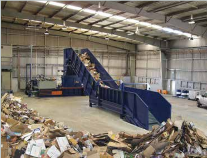
Below Ground with horizontal feed section and secondary horizontal sort section. 1800mm wide live width x 28 deg incline curved head section.
